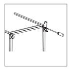
6. Unscrew and remove the bottom hinge pin with a flat screw driver, turn the bracket over and replace the pin.
